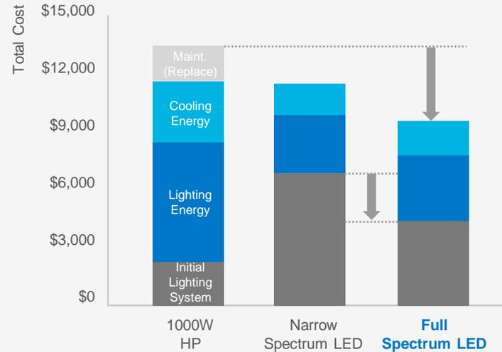
※ Unit Price : HPS (\$400 x 6ea), Narrow (\$1200 x 6ea), Full (\$780 x 6ea) / Lifetime : HPS (2khrs), Narrow (60khrs), Full (60khrs) / Electricity Rate : \$0.1 per kWh
