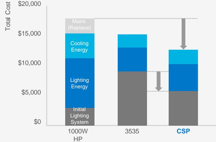
※ Unit Price : HPS (\$400 x 6ea), 3535 (\$1200 x 6ea), CSP (\$960 x 6ea) / Lifetime : HPS (2khrs), LED (60khrs) / Electricity Rate : \$0.12 per kWh
